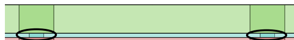
Figure 4: Cross view of a triple-layered stack, highlighting their anchoring points (black contours). The green and pink layers (top and bottom sheets) that compose the triple-layered stack present holes with a higher diameter than the blue layer (middle layer) allowing the formation of anchoring structures.
